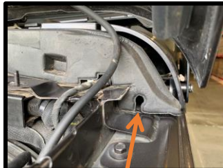
Pass cable through here
