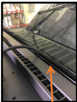
Tilt the windshield forward just enough to pass the cable down into the bottom of the windshield threshold
