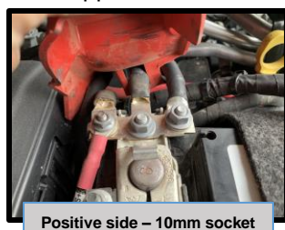
Positive side – 10mm socket
