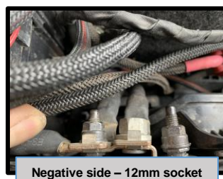
Negative side – 12mm socket
