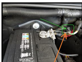
Negative side goes to a chassis ground
