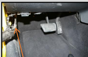
Look up into upper left side of firewall for the harness you just passed through
