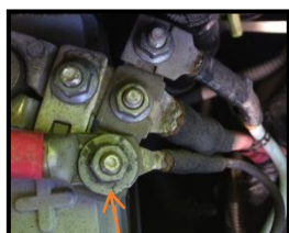
Positive side – 10mm socket
