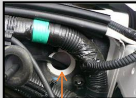
Use this grommet on upper right side of brake booster
